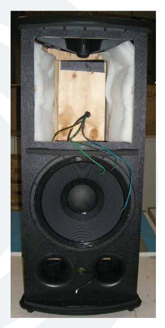
This is what it looks like with the grill and horn removed. See next page for further instructions and additional pictures on how to remove and replace the high frequency driver.
